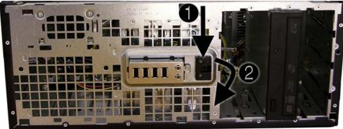
Figure 5-38 Removing the power switch assembly
